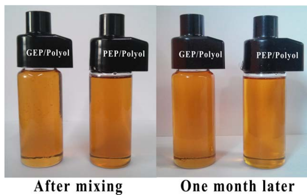
Figure 4. Photos of polyols with PAEPs. [Color figure can be viewed in the online issue, which is available at wileyonlinelibrary.com .]
